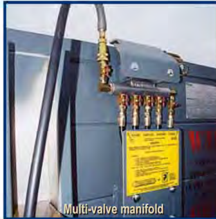
Pump can hose connection to manifold
