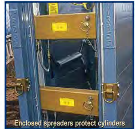
Spring contracts cylinder for removal
