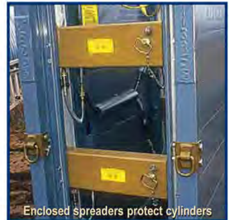
Spring contracts cylinder for removal
